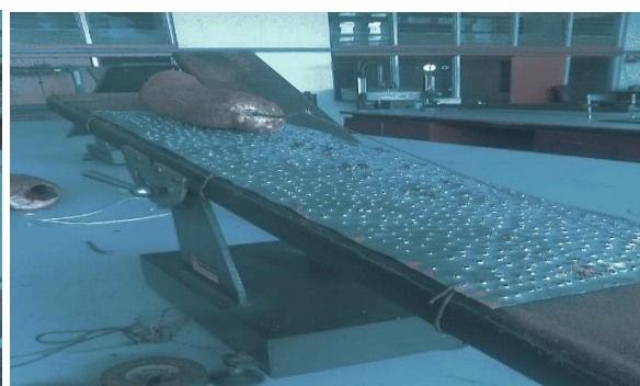
Fig. 5: Modified Friction Experiment Rig Showing string
