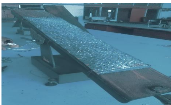
Fig. 4: Modified Inclined Surface for Friction Experiment
